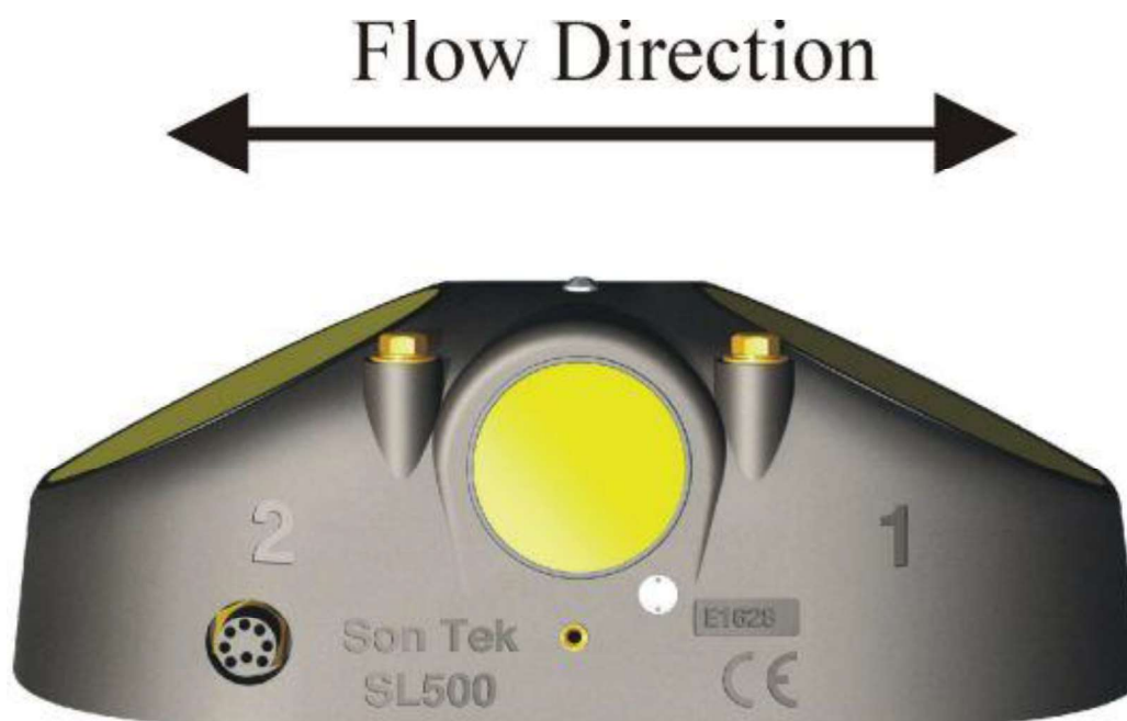
Figure 5-2. Argonaut-SL alignment with respect to flow direction
