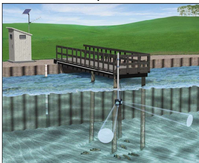
Figure 4-1. Typical Argonaut-SL Installation
