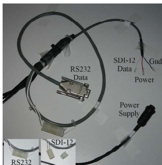
Figure E-1. Argonaut-SW Power/Communications Cable
