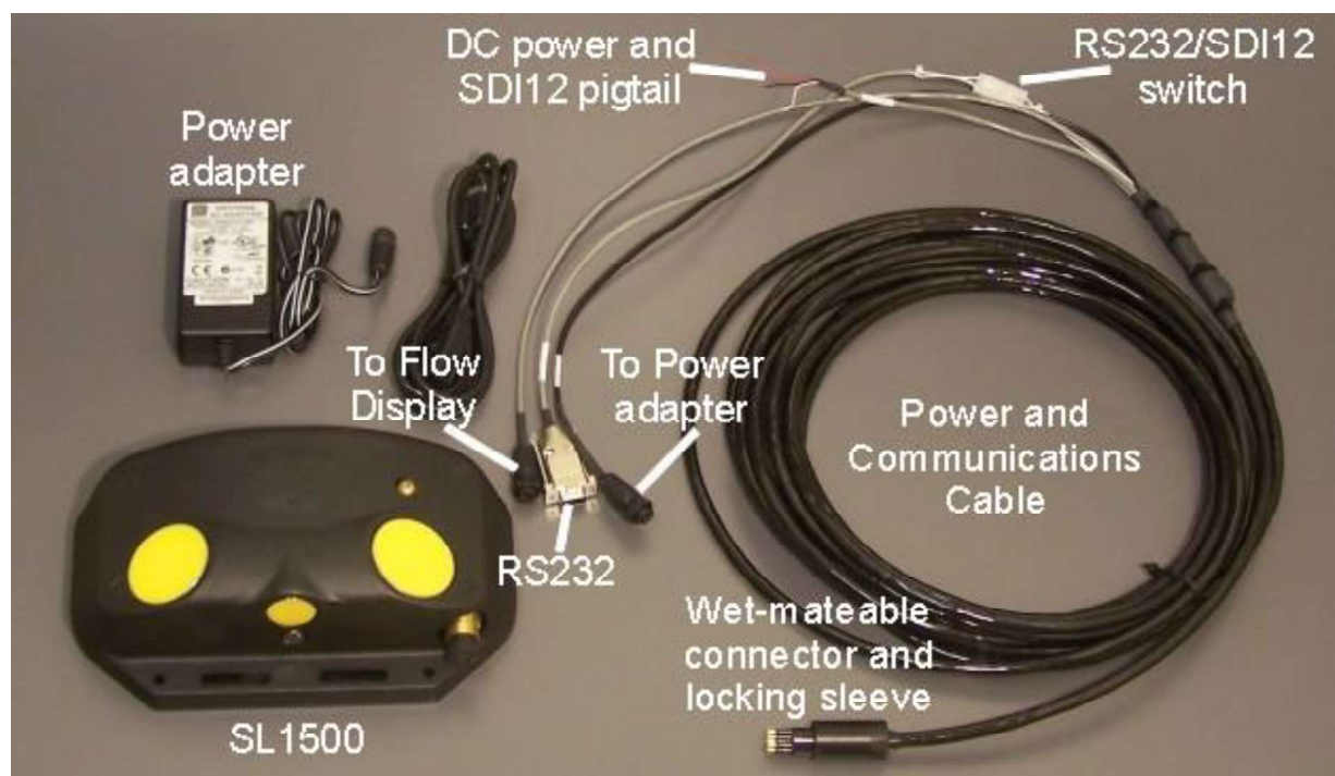
Figure 1-4. SL1500 with Standard Equipment
