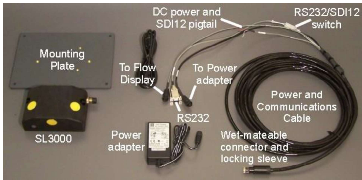
Figure 5-18. SL3000 with Standard Equipment
